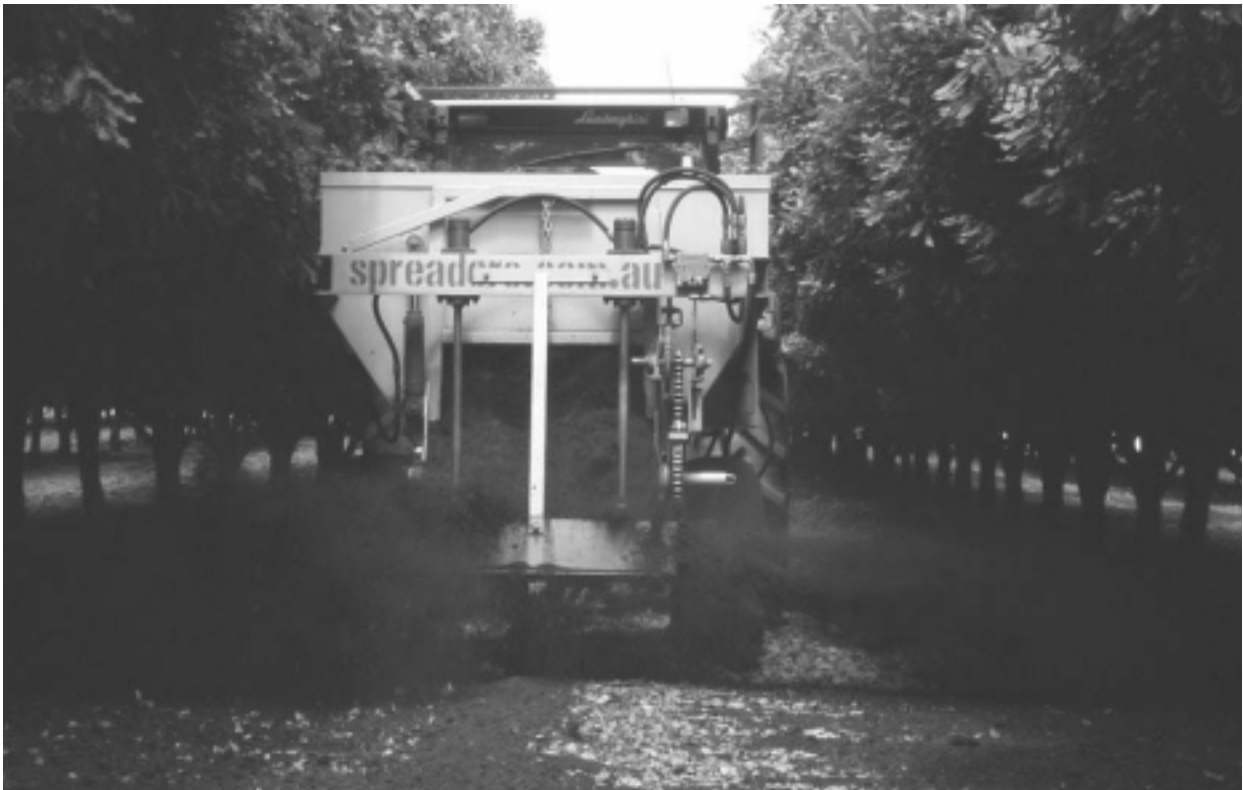
A twin disk spreader is effective for gaining an even coverage to a depth of 30 mm.
